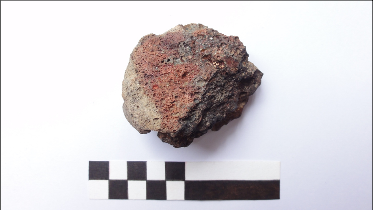
Fig. 3. Slag with adhering stone from C.229, lower surface
