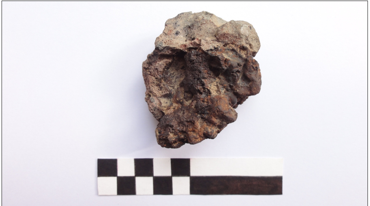
Fig. 1. Slag with adhering stone from C.229, upper surface
