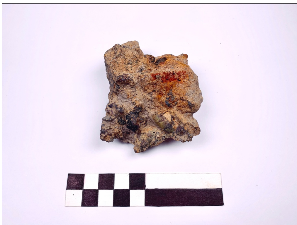
Fig. 1. Weathered smithing hearth cake from fill F13 within ditch F11
