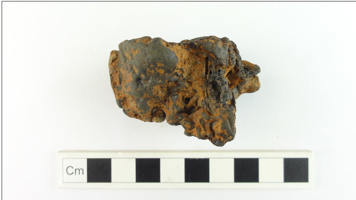
Fig. 1. Fragment of likely iron smelting slag from topsoil
